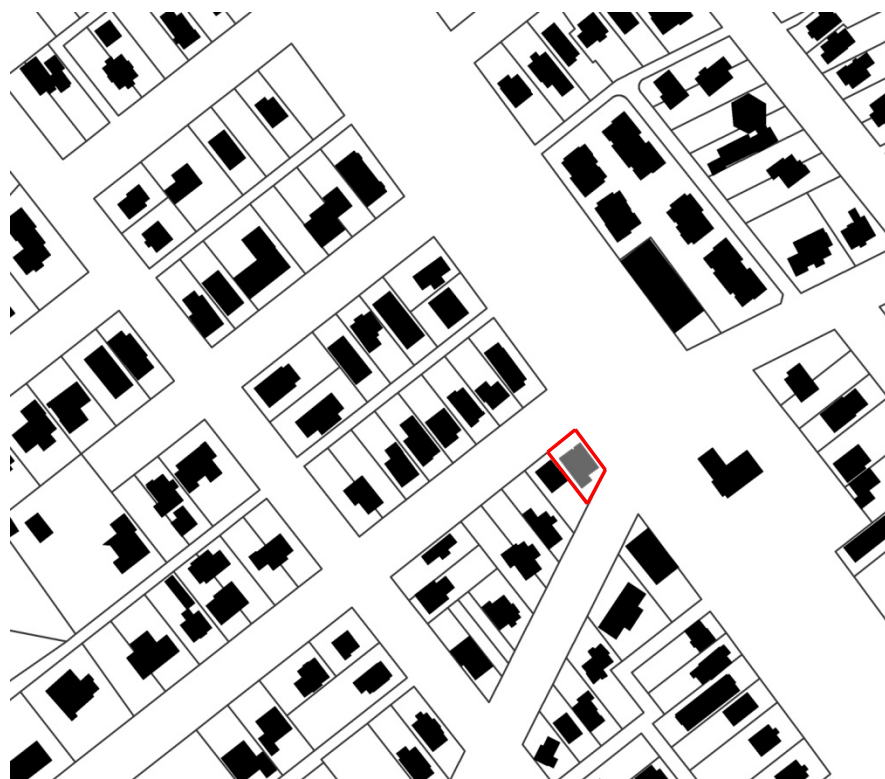
Figure 3. This image demonstrates the established development pattern in the surrounding neighbourhood. Existing building footprints are shaded in black, lots boundaries are shown in black outline and the proposed building footprint is shown in grey.
