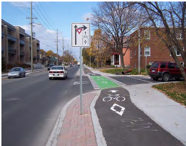
Figure 13 : Yield to cyclists when turning right sign
