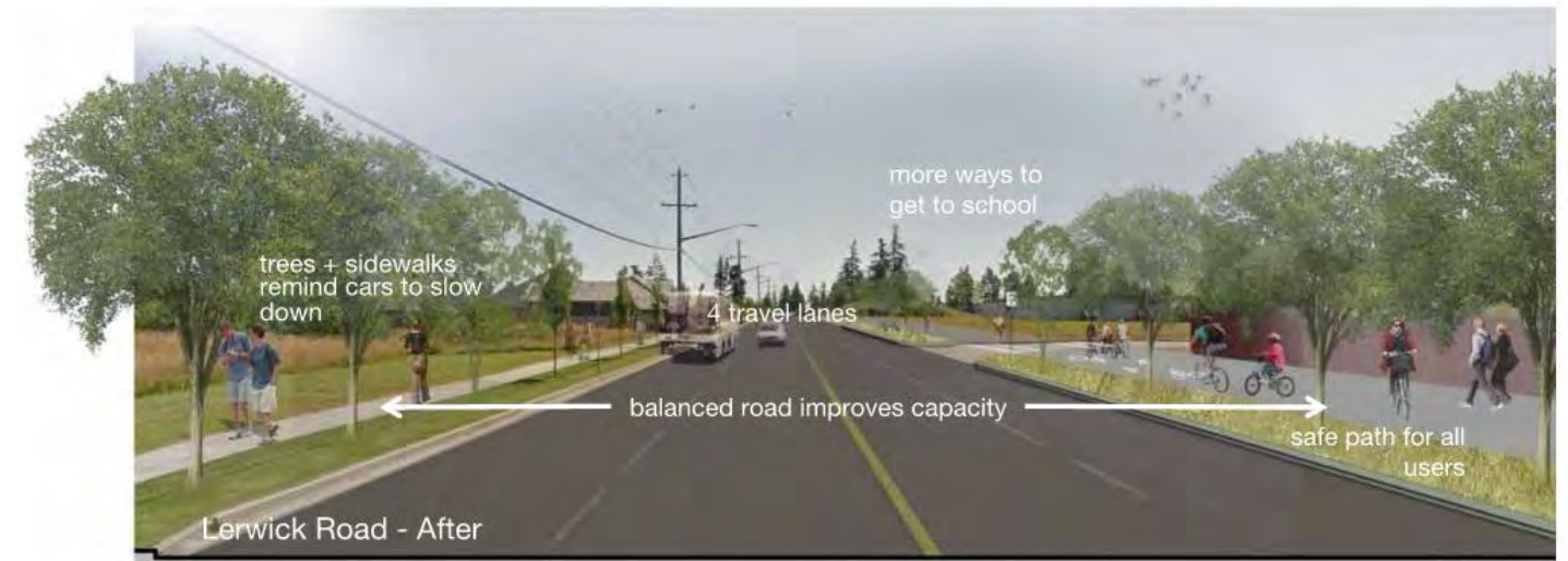
The provision of an additional travel lane on Lerwick Road improves conditions for motorists while a new off-road path creates a safer environment for walking and cycling.
