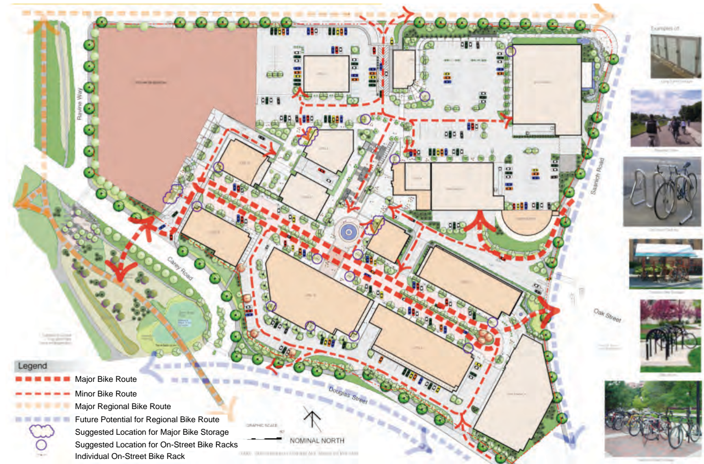
Short links and multiple access points promote high levels of on- and off-site pedestrian, cycling and vehicular connectivity in the commercial site plan for Uptown Centre in Victoria, BC
