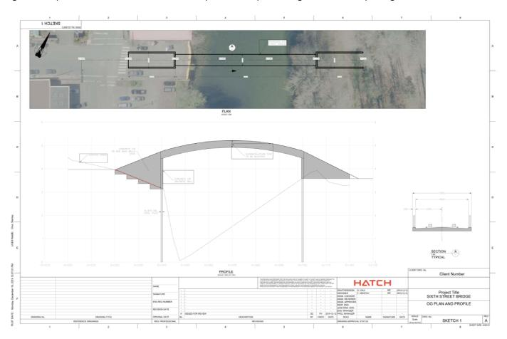
Figure 15: Bridge Embankments and Abutment Concept
