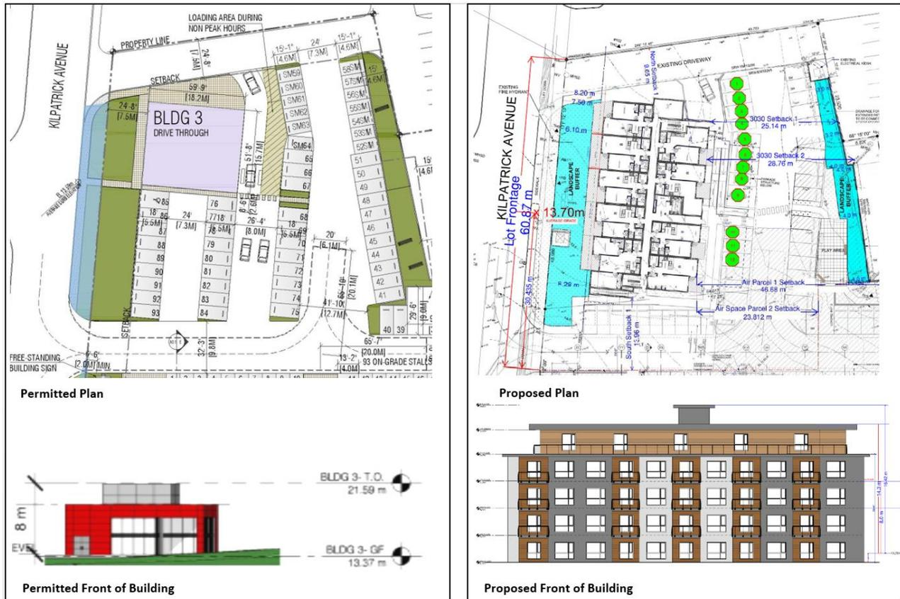
Figure 3: Subject Property Plan and Building Front as Permitted by CD-26 Zone (left) and as Proposed (right).
