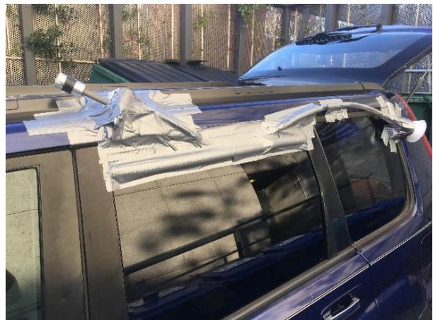
10. **Attach the air inlets to the instruments.**
