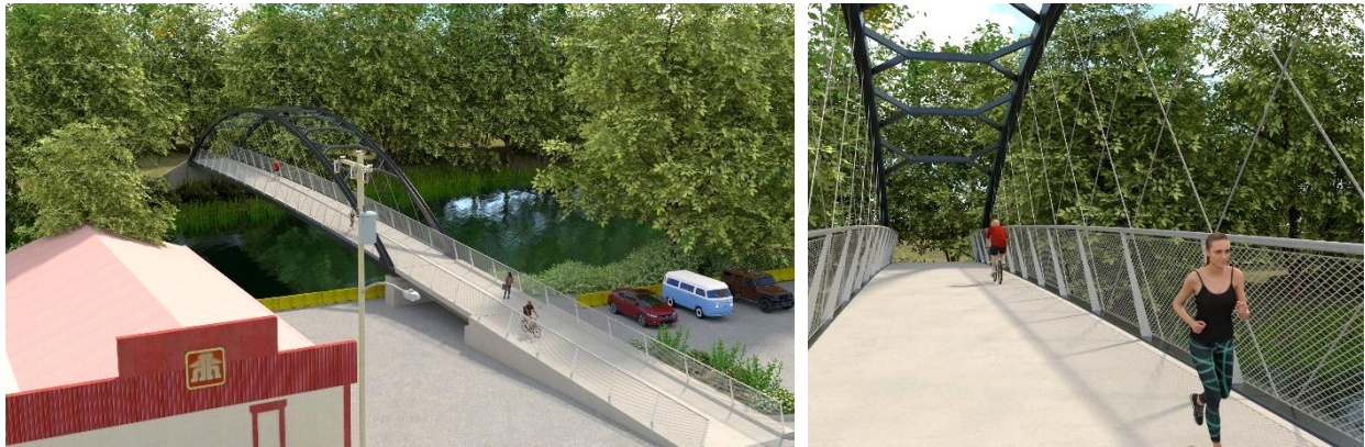
Figure 38: Renderings of network arch option at proposed project location
