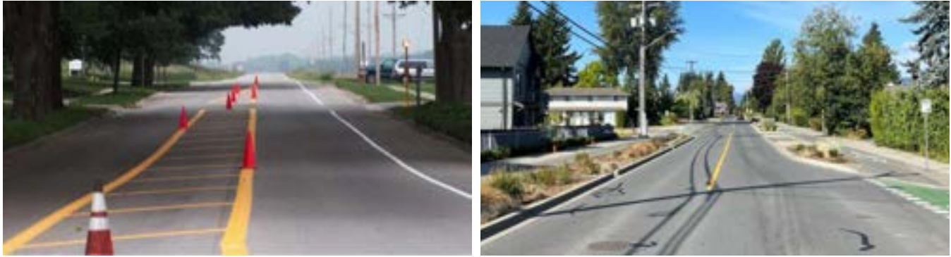
Figure 14. Sample Application of Lane Narrowing 22, 23
