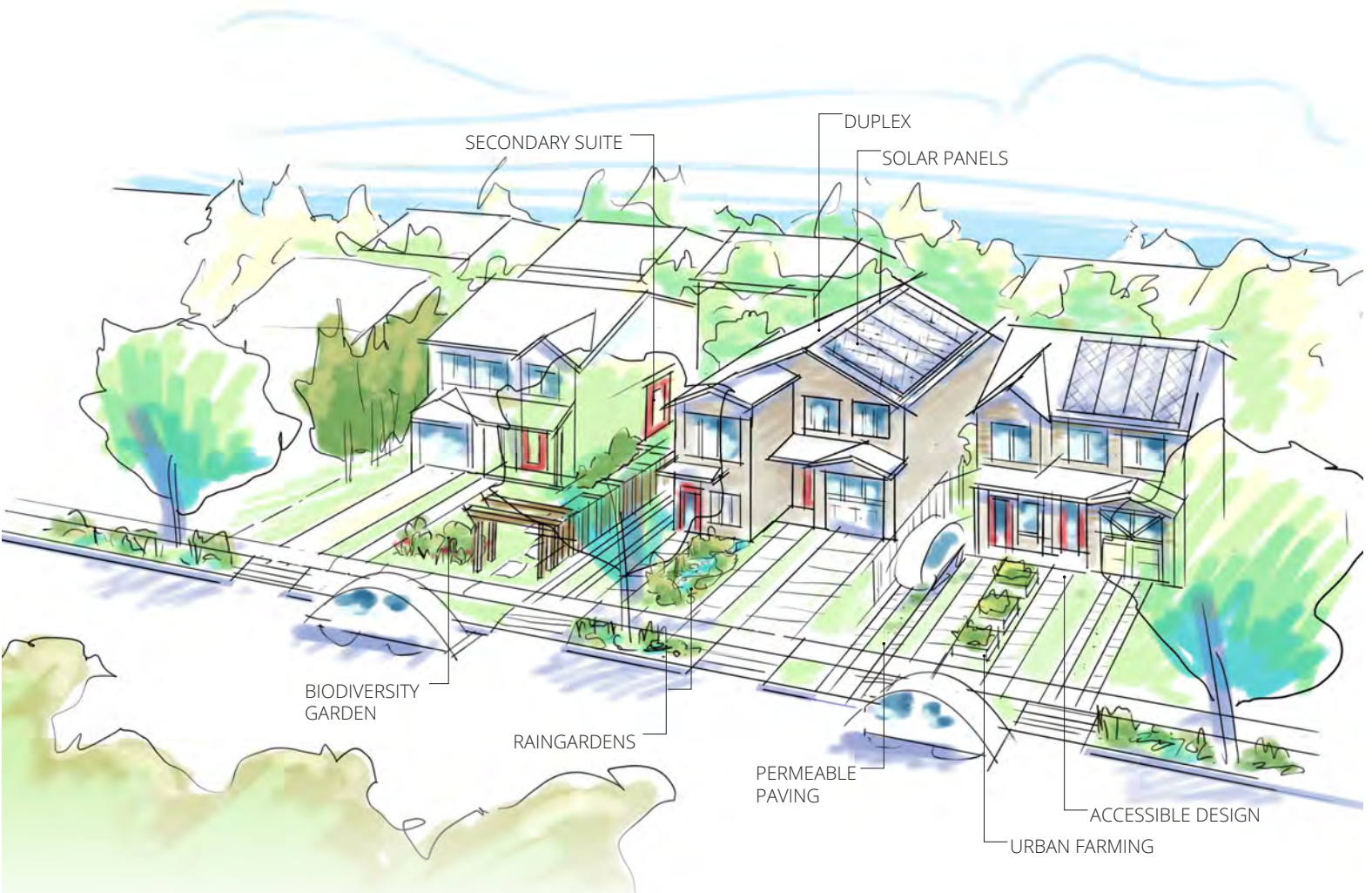
Figure B-6 Artist rendering showing infill and redevelopment on a residential street with climate-friendly design features.
