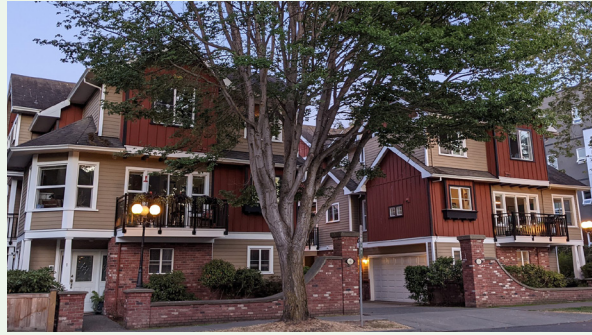
Example of a multi-residential building that has minimized the visual impact of parking by combining driveways (guideline 82) and facing garages away from the street (guideline 83).
